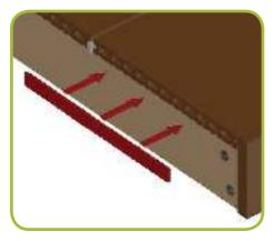
PAVEEZZI Composite End Caps are an alternative to the PAVEEZZI Composite Finishing Board. These are to be inserted into the end of each PAVEEZZI Composite Decking board.
