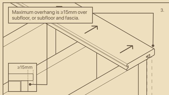
After installing the first board successfully, use the following method for all subsequent boards to complete the deck. Do not pre cut boards to size. Cut boards with an extra 10-15mm length, this will allow you to use a track saw to cut all the ends to size at once when ready to finish. This will minimise any variation in gaps due to temperature differences.
