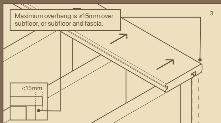
After installing the first board successfully, use the following method for all subsequent boards to complete the deck. Do not pre cut boards to size. Cut boards with an extra 10-15mm length.
